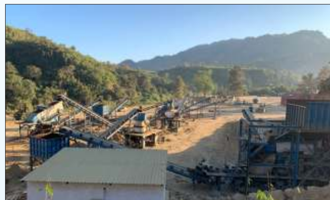
Installation of Stone Crusher at Camp-1 km. 0+000 ( Construction of Two Lane Road on NH Specifications from Paletwa to India-Myanmar Border (Zorinpui) from km 0.00 to km 109.2 in Chin State of Myanmar)
