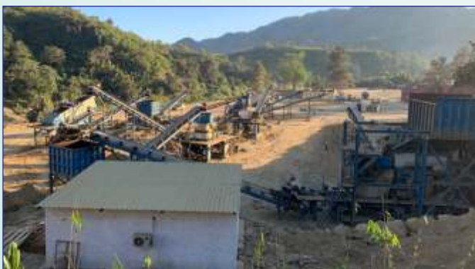
Installation of Stone Crusher at Camp-1 Km. 0+000 (Construction of Two Lane Road on NH Specifications from Paletwa to India-Myanmar Border (Zorinpui) from km 0.00 to km 109.2 in Chin State of Myanmar)
